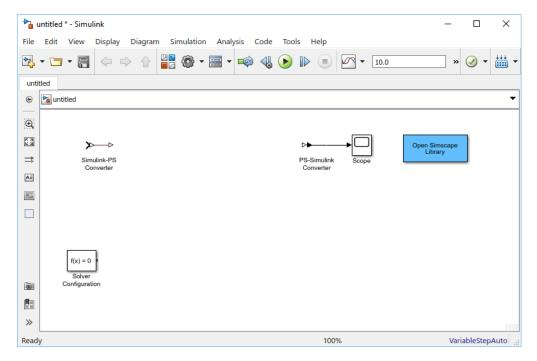
By default, the model name is not specified, the model contains a Solver Configuration block, a Simulink-PS Converter block, and a PS-Simulink Converter block connected to a Scope block. The default solver is VariableStepAuto. Double-clicking the Open Simscape Library block opens the main Simscape library.
