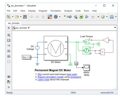
7 Connect the blocks as shown in the following illustration. To rotate a block, select it and press **Ctrl+R**.
