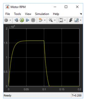
**3** Try varying the load torque to find the maximum torque at this reduced voltage. Open the Step Input subsystem and double-click the Step source block. Enter different final values for the input signal and rerun the simulation.
